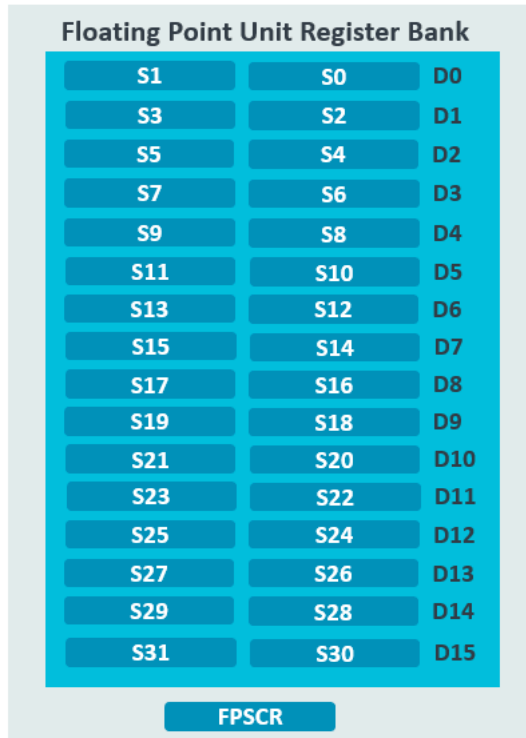
Figure 5-8: FPU Registers
